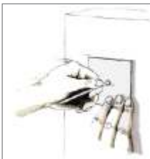
Place the hanger in the required position and press the base against the surface to be insulated
